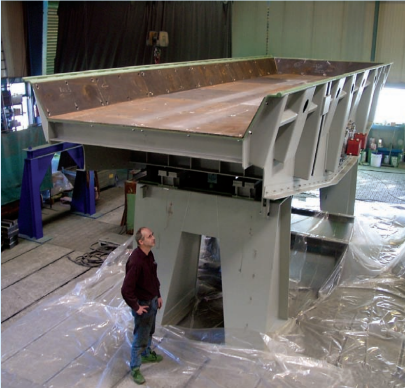
Shredder Conveyor 2,600 x 8,000 mm. Trough dimensions can be varied according to shredder size and performance requirements
