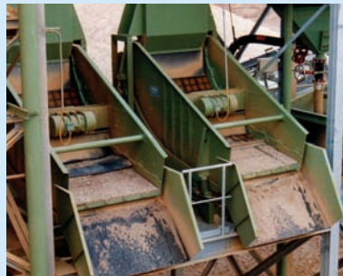
Drainage 200 m 3 , 1,500 x 3,600 mm, stone/sand
