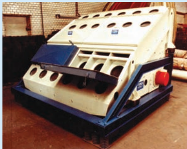
Compact design, double-decker screening machine
