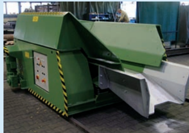
Charging machine, compact design, 3 t bin volume, height overall 1,250/1,500 mm
