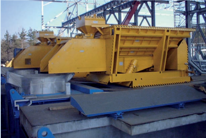
Charging machine with additives container
