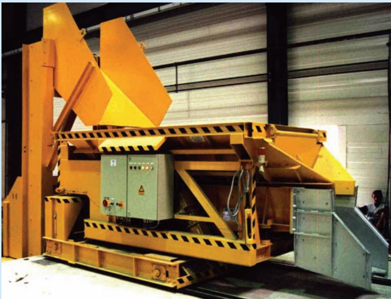
Charging machine 2 m 3 with lifting and tilting equipment
