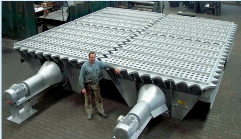
Shake-out grid 6,300 x 6,300, load-bearing capacity up to 40t (single loads up to 15t/screen)
