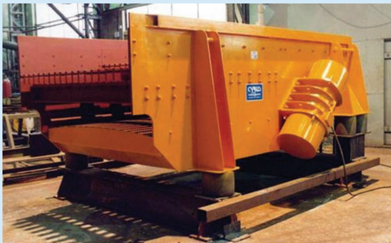
Special separator screen 1,600 x 4,000 mm incl. separation
